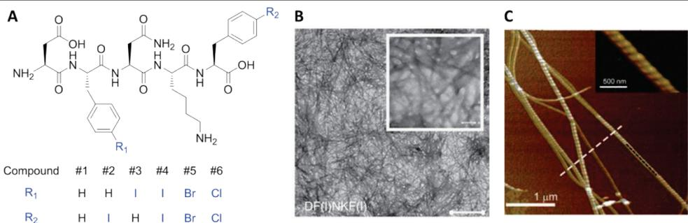
**Figure 2** – Chemical structures of the first series studied (A) and TEM (B) and AFM (C) images of compound #4, confirming the amyloid structure of the peptide self-assembly.<sup>[3]</sup>
